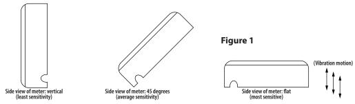
\*Note: All equipment, vibration levels, and vibration direction are unique. This meter is designed to filter out most road travel and count actual equipment run time, but may require trial and error per the application.
